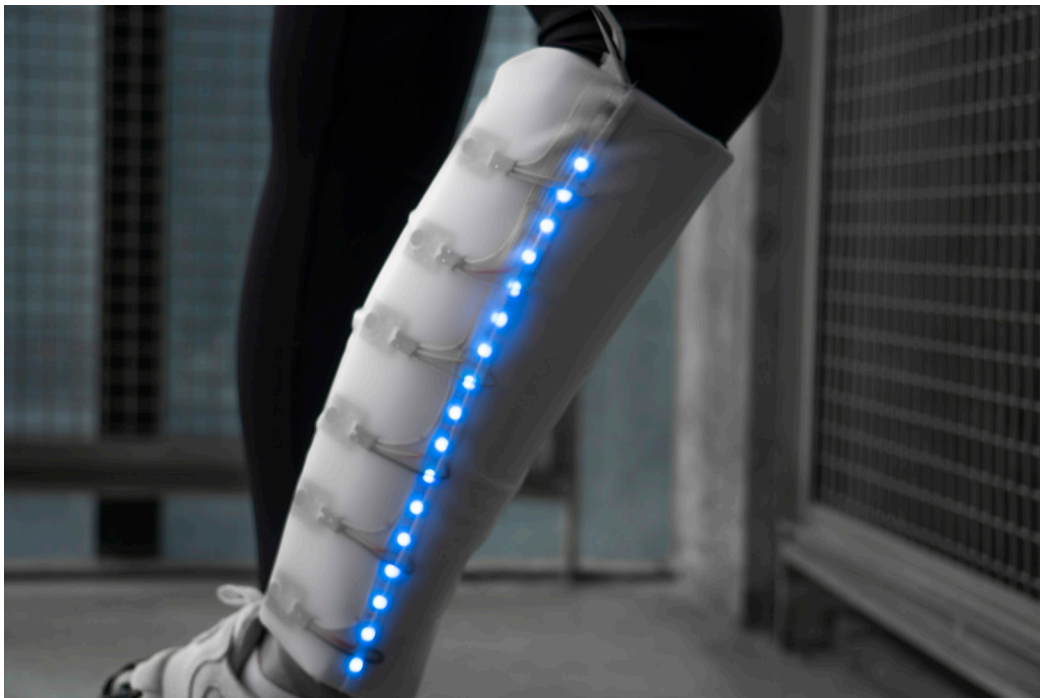
Figure 6. New Instinct The project is a collection of two wearable devices that use electronic components to let the wearer experience the senses of animals: the first device is a shin piece that mimics the ability of oysters to perceive the sea tides. A series of vibration motors placed inside the piece turns on or off in succession to indicate the variation of sea level.
