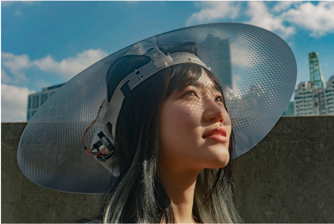
Figure 7. New Instinct. The second device replicates birds' capacity to navigate using the magnetic field of Earth. A harness holding a stepper motor rotates a visor cap according to the input of a compass sensor. When the wearer moves, the motor rotates to keep the visor cap aligned to the north.
